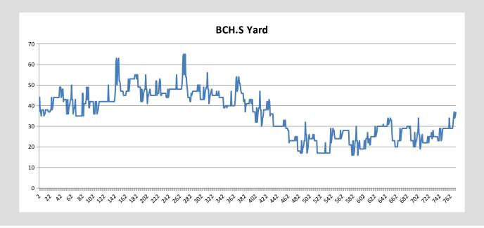
One of the most useful plots is the number of cars at a track or station over time. This gives a simple insight into how well the layout is *balanced*.
