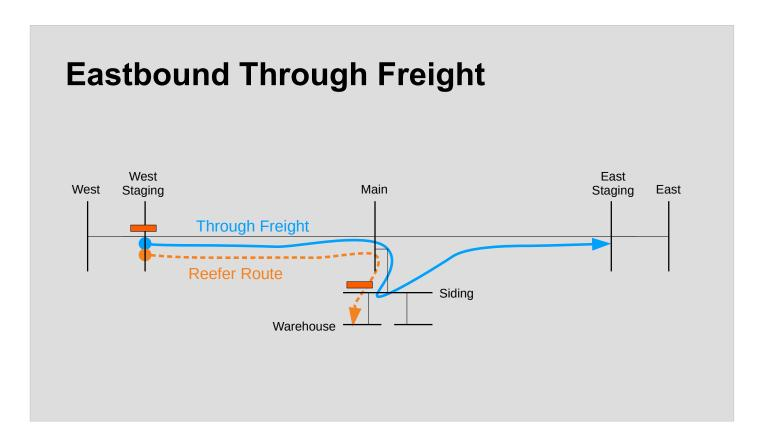
A Through Freight will usually not visit individual industries but just switch a track in town, such as the Siding. The Siding is along the car's route, so the Through Freight can advance the car, but not all the way to its destination.
