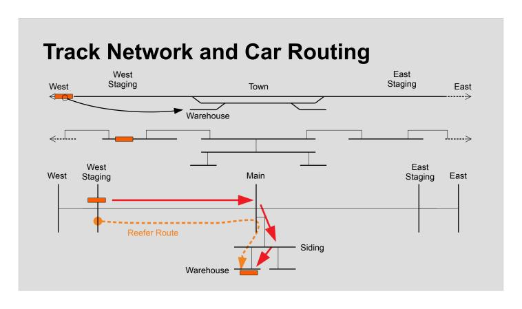
A *Network* of interconnected *Tracks* is used to decide the routing of cars across the layout. This is not specified by the user, but is calculated by analysing the *connections* between tracks.
