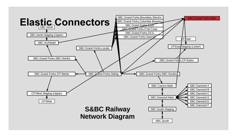
Track placement is left to the user to do in LibreOffice because the program has no way of knowing how the tracks should be arranged. The locations of the tracks are maintained though updates, but the connections are all completely redrawn each time the diagram is updated.
