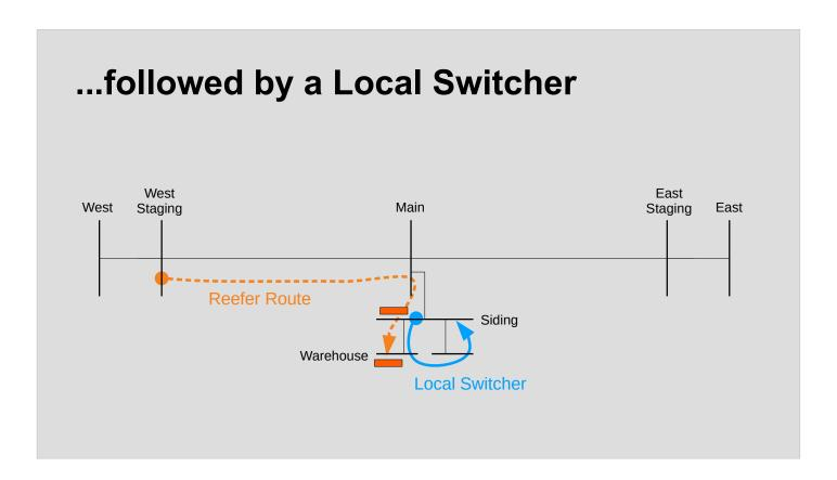
A Local Switcher would be responsible for servicing the local industries by delivering and picking up cars, and collecting them for pickup by a Through Freight.
