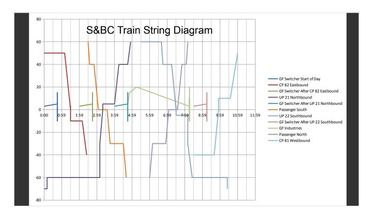
The train timetable data can be processed into a graph that shows the relative train positions over time. This is known as a *String Diagram*.
