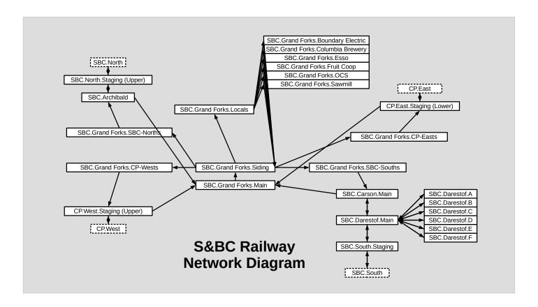
The track and connection data can be processed into a basic *network diagram* that makes it easy to visualize how cars can flow over the layout.
